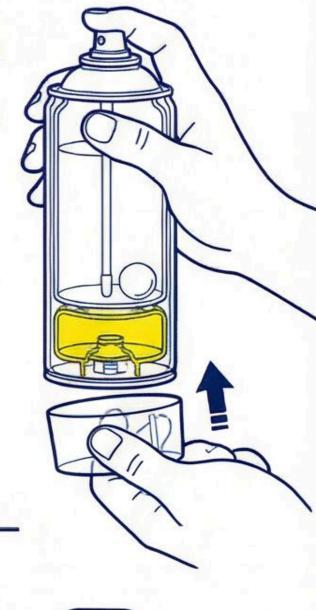
B. ACTIVATE HARDENER PRESS BOTTOM ACTUATOR ON FLOOR
